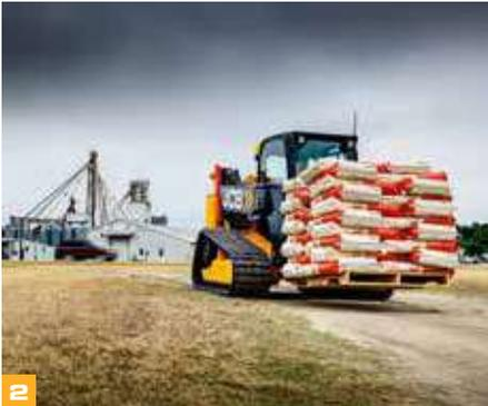
1 The ability to lift over 13 feet allows you easily and quickly load trucks without needing a ramp.
