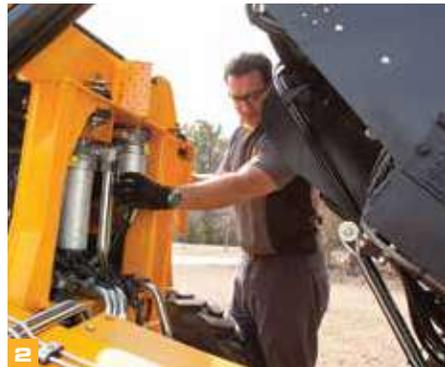
1 Large rear service door provides easy access to all daily maintenance points and engine bay. All daily checks and greasing can be done at ground level.
